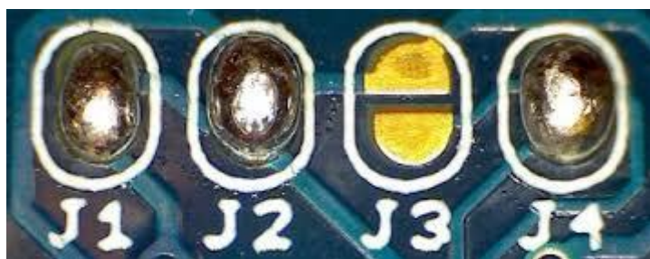
Figure 4 Solder Jumper NO (“normally open”)
